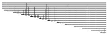
Size of circuit is proportional to number of low-level bit-operations in all execution paths of adder.
